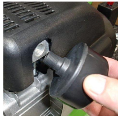
Remove the cap and screw air filter by hand
